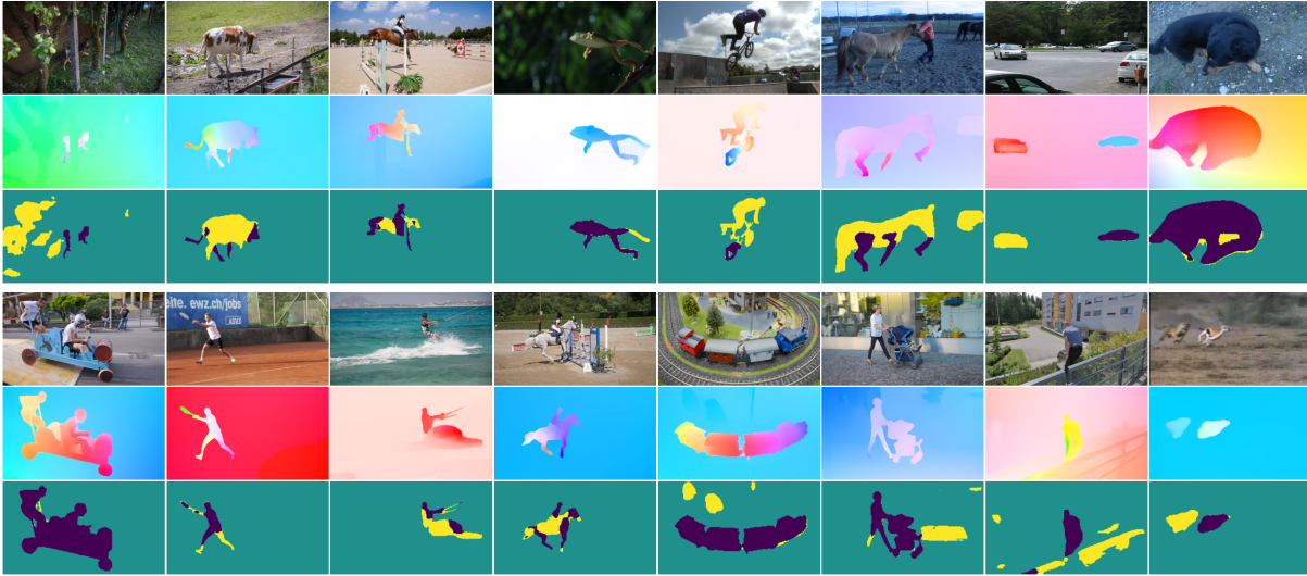
Figure 3.8 – Results obtained with our method using four masks ( K = 4 ), but the network may not necessarily use all the four masks. Two groups of results. For each group, the first row depicts one image of the video, the second row contains the optical flow input represented with the usual HSV color code, the third row displays motion segments (given by layers that are not necessarily connected) with one colour per segment. Samples are drawn from the different datasets.
