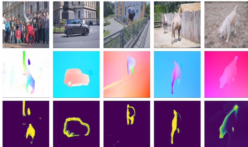
Figure 6.3 – Results regarding the task of independent motion detection on DAVIS2016 dataset. From left to right: breakdance , car-roundabout , parkour , camel , dog videos. From top to bottom: RGB frame, optical flow field (HSV color code), predicted salient motion mask.
